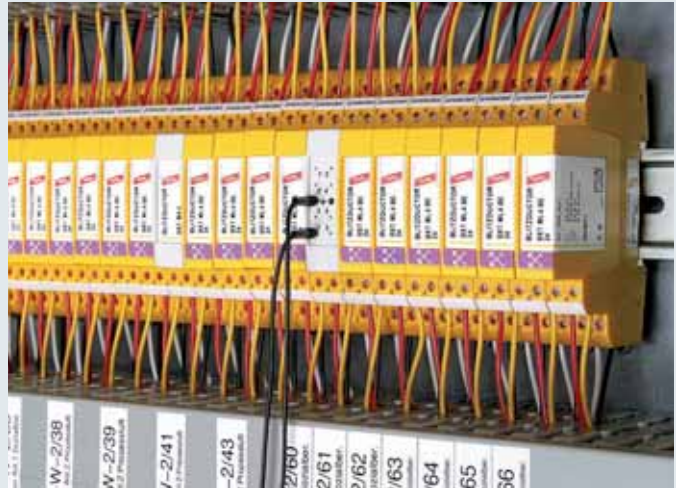
Pluggable multi-pole universal lightning current/surge arrester for use in IT systems. The SPD modules with integrated LifeCheck allow for quick testing of SPDs without contacting by means of a portable reading device or stationary condition monitoring system. SPD module and base part have to be ordered separately.
