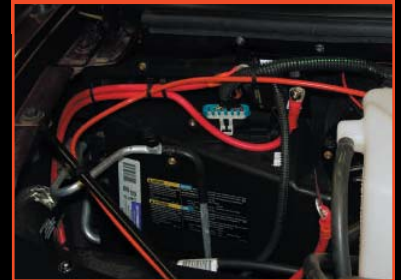
The red Firetrace Detection Tubing (pictured above and below) can be run across all potential hazard areas, ensuring detection is close to the most probable fire sources.
